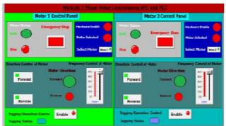
Fig.7 SCADA Control Screen when induction motor runs in forward direction
