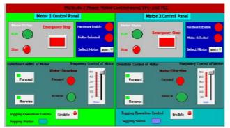
Fig.9 SCADA Control Screen when induction motors in reverse and forward direction
