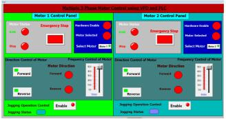
Fig.6 Initial SCADA Control Screen for induction motor
