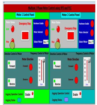
Fig.5 SCADA Control Screen when protected with password
